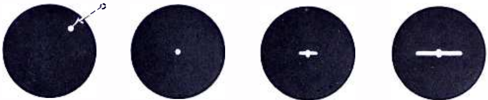
Fig. 7—A nightfighter airplane radar image. Center of image is center of gunfire. Length of simulated wings proportional to nearness of the target.
